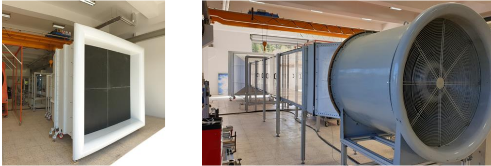
Figure 4.1 Open return boundary layer wind tunnel facility at Center for Wind Energy Research (RÜZGEM) at the Middle East Technical University (METU)
