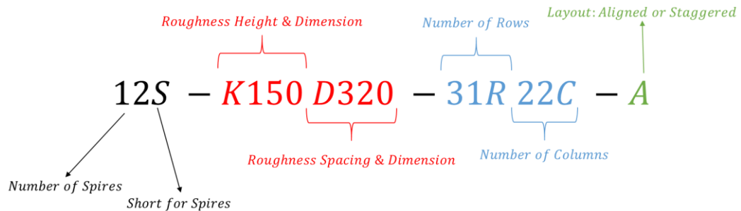
Figure 3.12 Terminology for spires and roughness elements
